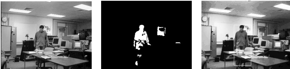
Figure 9.1: (Left) A person appears in a formerly unoccupied workspace. (Center) Image subtraction reveals changed regions where the person occludes the background and at the door and a CRT. (Right) The change due to the person is deemed significant while the other two are expected and hence ignored. (Images courtesy of S.-W. Chen.)
