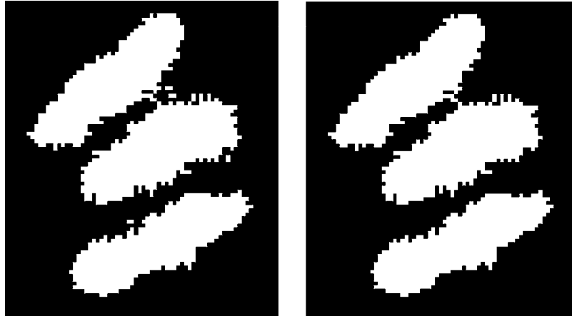
Figure 5.6: (Left) Bacteria image of Figure 5.5 after salt-and-pepper noise was removed using a 4-neighborhood and (right) image with small components removed. Original image courtesy of Frank Dazzo.
