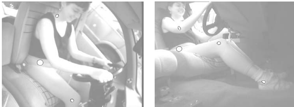
Figure 13.1: Two images of the driver of a car taken from two of four onboard cameras. A multiple camera measurement system is used to compute the 3D location of certain body points (identified by the bright ellipses) which are then used to compute posture. (Images courtesy of Herbert Reynolds, Michigan State University Ergonomics Lab.)
