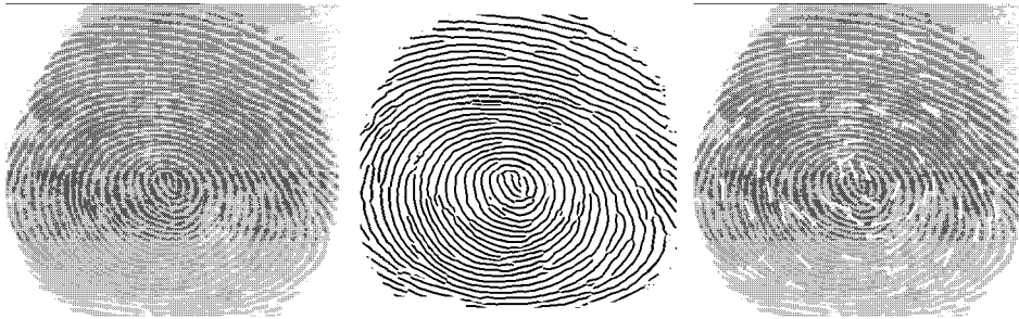
Figure 5.2: (Left) Original sensed fingerprint; (center) image enhanced by detection and thinning of ridges; (right) identification of special features called “minutia”, which can be used for matching to millions of fingerprint representations in a database (contributed by Shaoyun Chen and Anil Jain).
