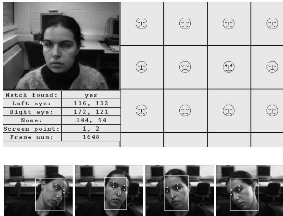
Figure 9.17: Tracking of the eyes and nose of a workstation user enables movement of the cursor without using the mouse. (Top) Face pose determines selection in menu. (Bottom) A sequence of face images showing tracking of the eyes and nose. (Images courtesy of Vera Bakic.)
