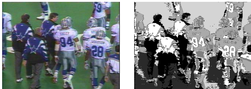
Figure 10.1: Football image (left) and segmentation into regions (right). Each region is a set of connected pixels that are similar in color.
