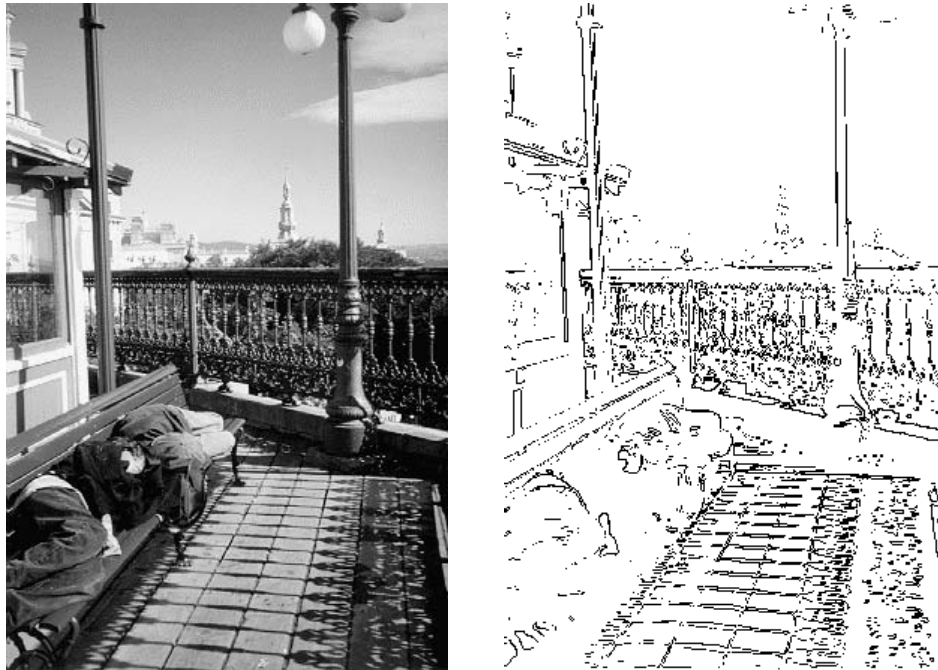
Figure 12.10: In Quebec City above the cliff above the great St Lawrence River: (left) image showing many depth cues, (right) result of Roberts edge operator followed by thresholding to pass 10% of the pixels.
