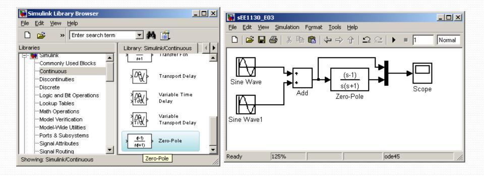
• When studying Filter Theory you will learn that the roots of the numerator (called zeros) must be  $s=2\pi60j$  where 60 is the frequency to eliminate at the output.
