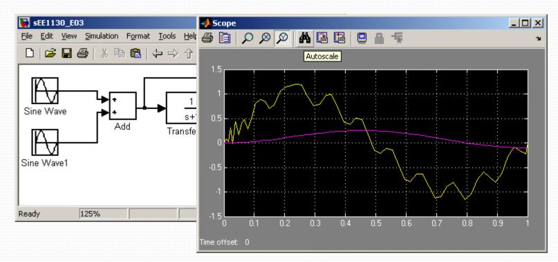
• Somehow we cleaned the signal, but we need to amplify its gain by a factor of 4. We open the transfer function and set 4 the numerator to do this.
